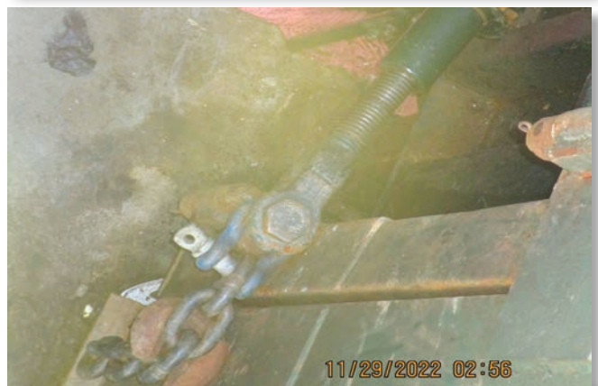
The household/garbage waste container and the compactor were connected. Due to the two items being connected when the rollback truck was retrieving the container, the container shifted towards the retention wall resulting in employee 1 being pinned between the retention wall and the container.
