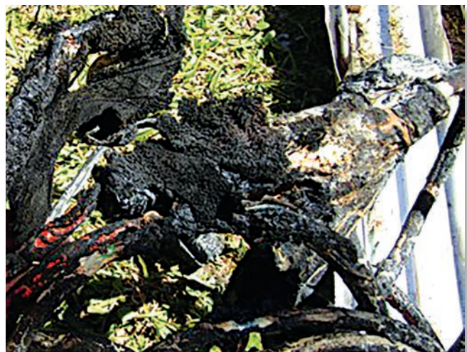
Glove melted around the electrical cord.
