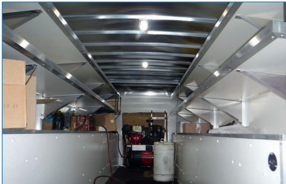
Photo showing the inside of the service truck body with the compressor installed forward of the rear entry doors closest to the cab.
