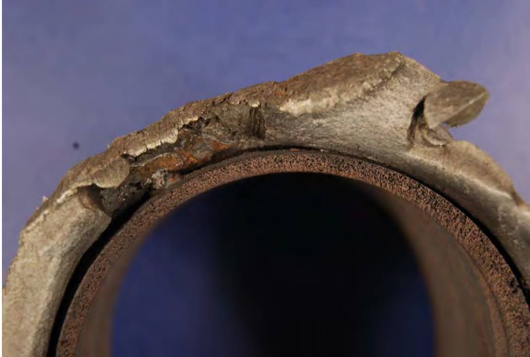
30. Close-up of Tube 10 showing poor weld
