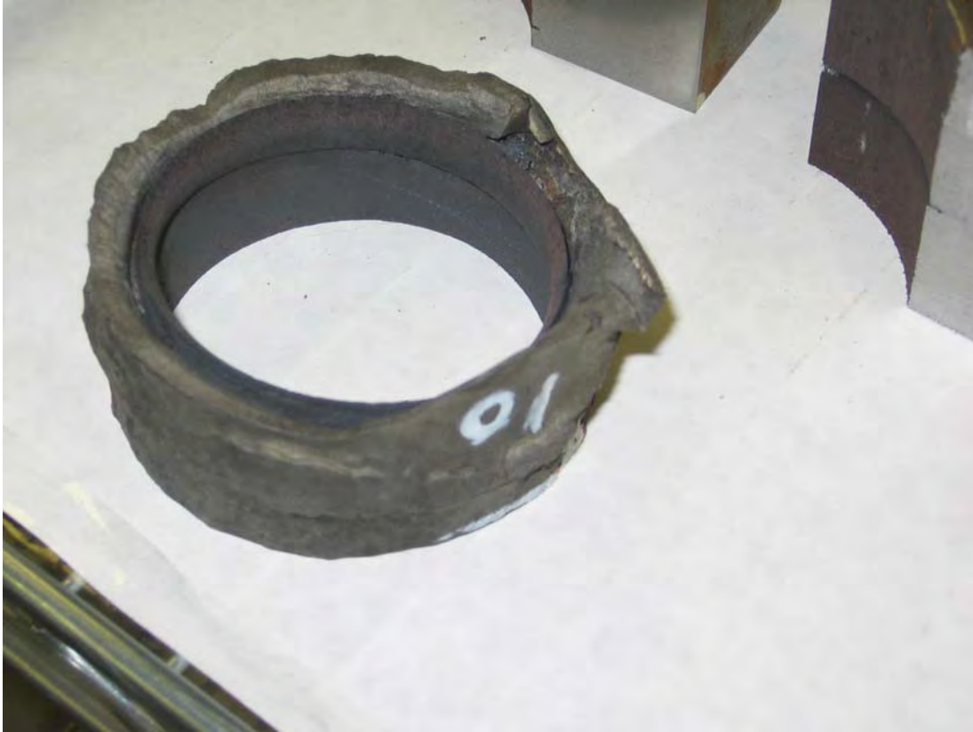
38. Cut away of Tube 10 stub (with bad weld)
