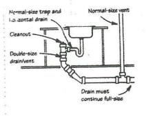
Figure 3. A double-sized single fixture wet vent provides enough makeup air to allow the drain to flow freely.
