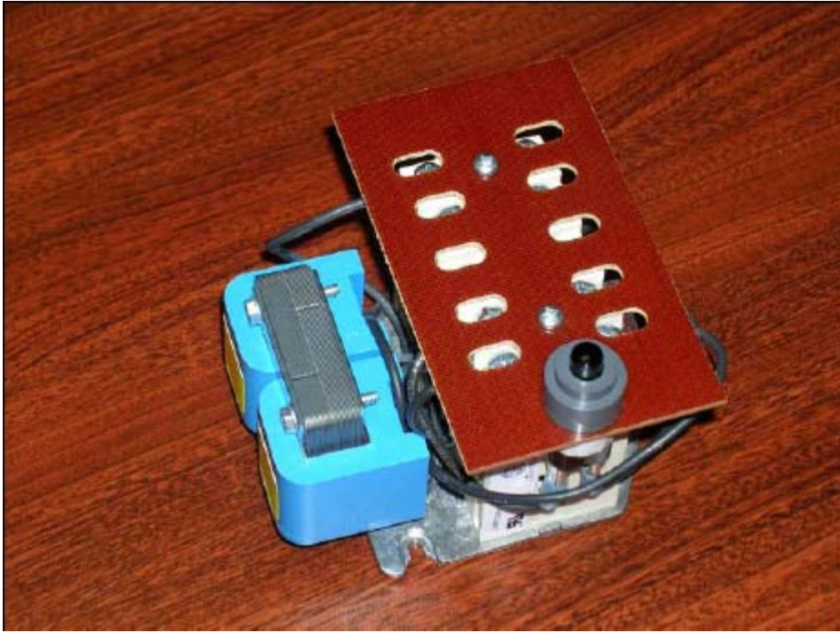
Photo #17a –1c1d0a (Proper Relay with Manual Reset)
